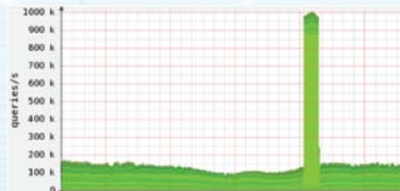
August, 2010, CommunityDNS' Hong Kong node experienced 2 hour traffic spike. This node comfortably handled over 863,000 queries per second.
